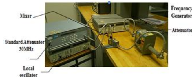
Fig. 2: Realization of the Substitution intermediate frequency
