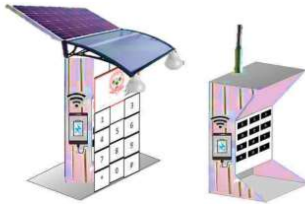
Figure 2-b: wifi station & solar charger.
